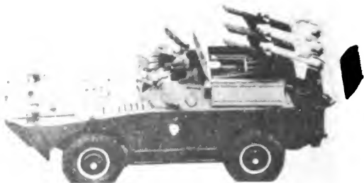
Figure 6-37 AT-2 SWATTER. SWATTER missiles appear in a quadruple mount on a modified BRDM. Shown here is the launcher raising sequence.
